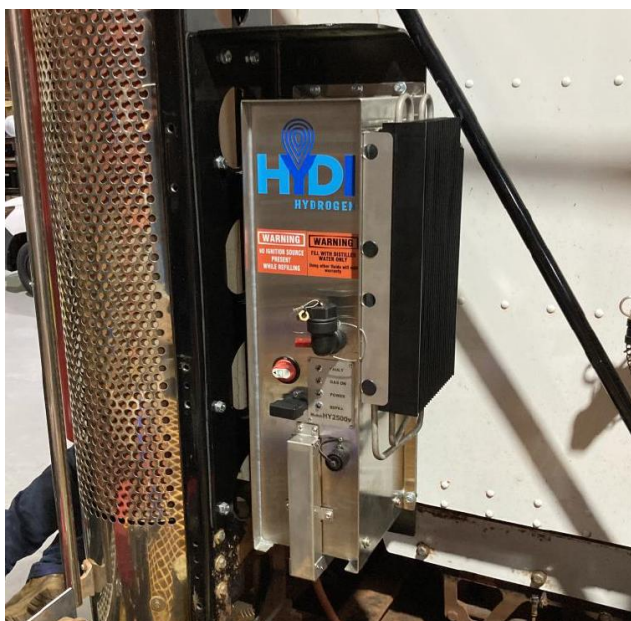
Figure 4: HY2500 vertical mount with custom bracket
